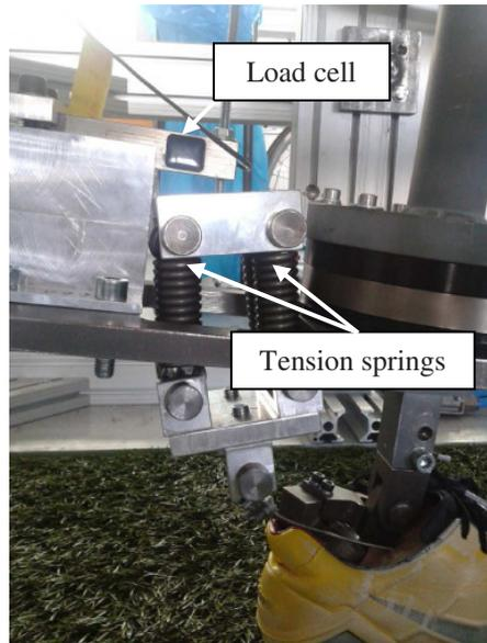
Fig. 3. New Achilles tendon model
