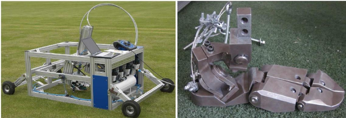
Fig. 1. Custom made test jig TrakTester (left) with metal skeleton of the original foot model [3]
