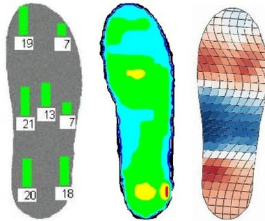
Fig. 4. Pressure distribution at the original foot model (Parotec, left, Grund 2011), the modified model (Pedar-X, middle) and the inflexible model (OpenGo, right)
