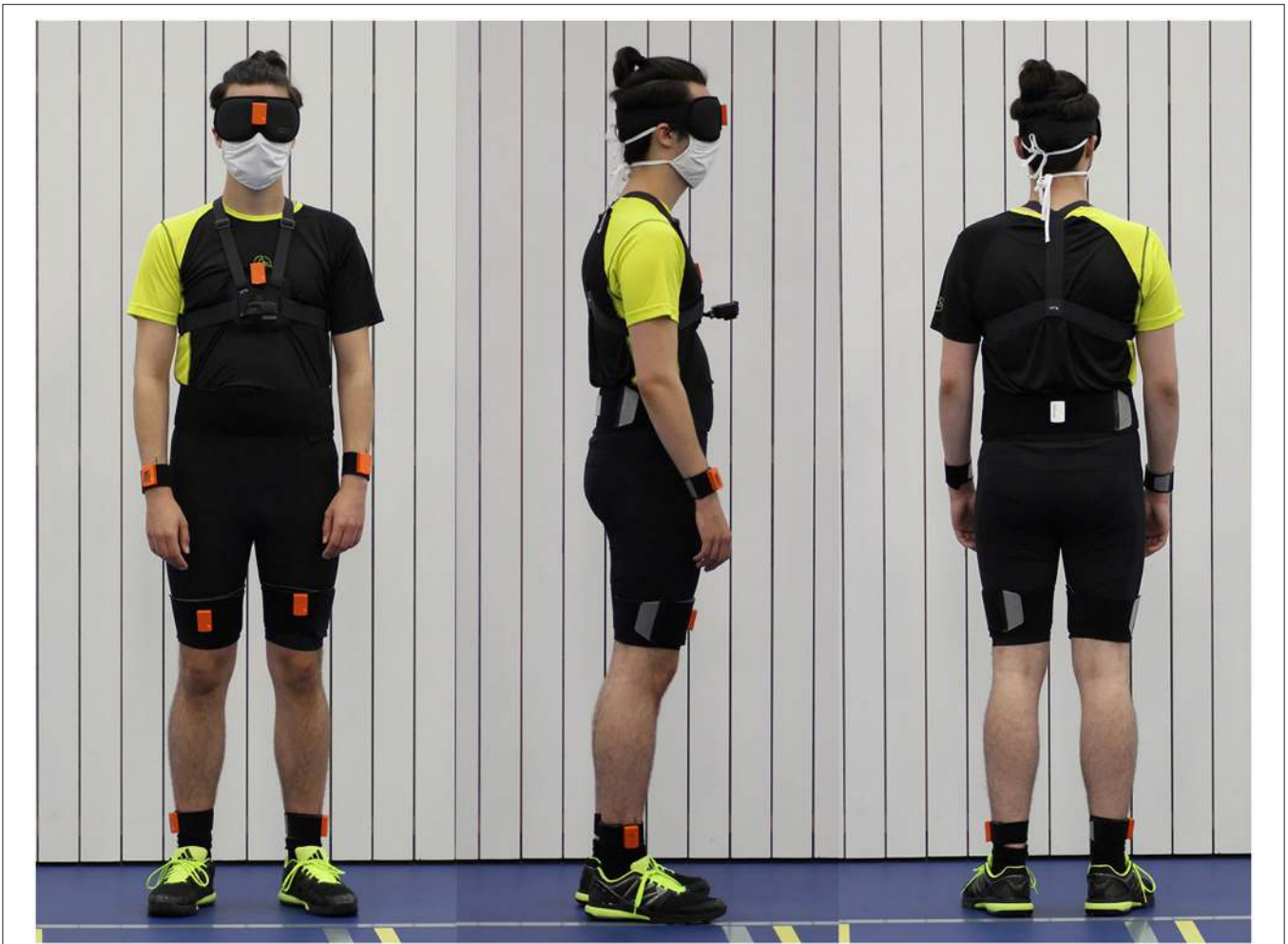
FIGURE 1 | The fully-equipped participant during the study; 9 IMUs (MTw Awinda, Xsens Technologies B.V., Enschede, Netherlands) were attached to the subject with Velcro® patches and bands at both ankles, both thighs, lower back, chest, both wrists, and at the forehead. Sensory shoe insoles (Insole3, Moticon ReGo AG, Munich, Germany) were laid in the subject's own shoes. Additionally, the subject wore a GoPro Hero 6 on a chest mount (GoPro Inc., San Mateo CA, USA), a sleeping mask and earmuffs.
