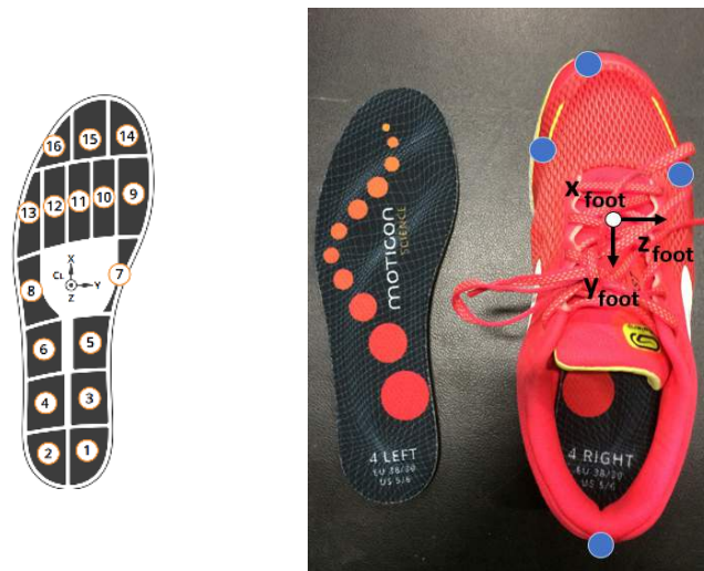
Figure 3. Shoe equipped with instrumented insoles and markers enabling the construction of the foot reference frame.
